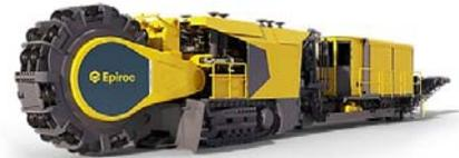
Produced by Epiroc (formerly known as Atlas Copco), this project is developing a new electrically powered mechanized mining machine which uses a large diameter rotating cutter head to fracture rock and direct it onto an under-mounted transfer belt that carries muck to where it can be handled at the back end of the machine.
