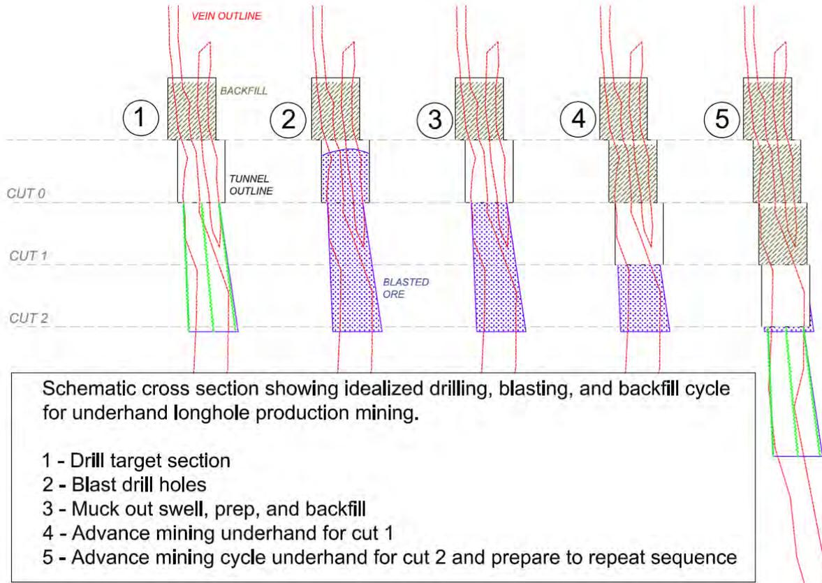
**Figure 13-3: Underhand Closed Bench Mining Method Schematic**
