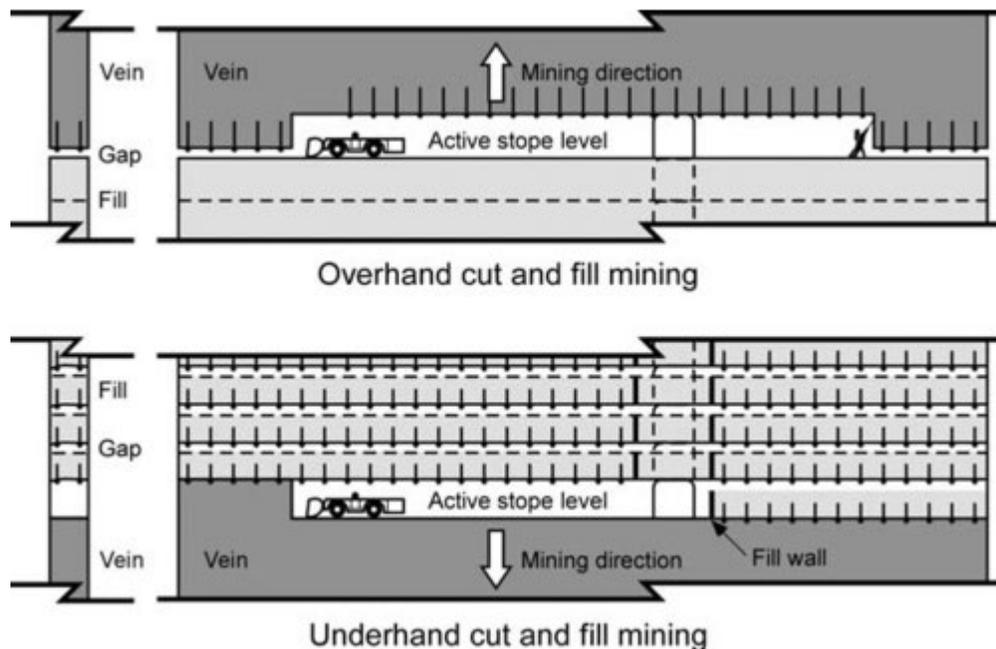
**Figure 13-2: Mechanized Overhand and Underhand Stoping**
