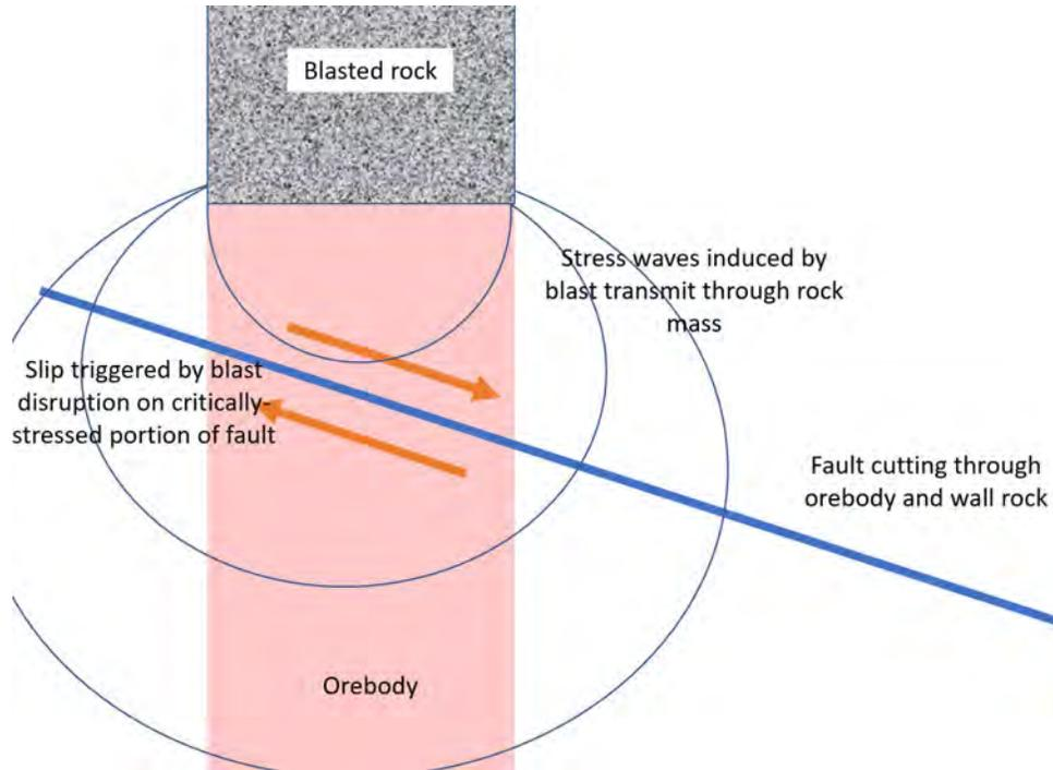
**Figure 13-4: Conceptual Fault-Slip in UCB Cross Section**
