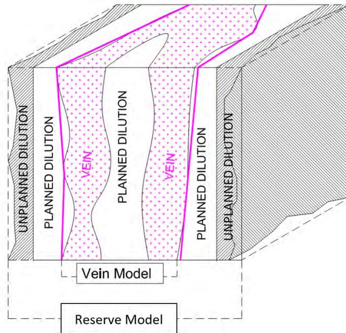
**Figure 12-1: Dilution Schematic**
