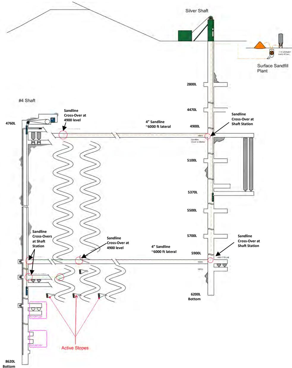
Figure 13-5: Backfill Schematic
